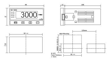
▲ Caution: Maintenance and to ensure the safety of the device if you add a space to more than 125min size is recommended.
